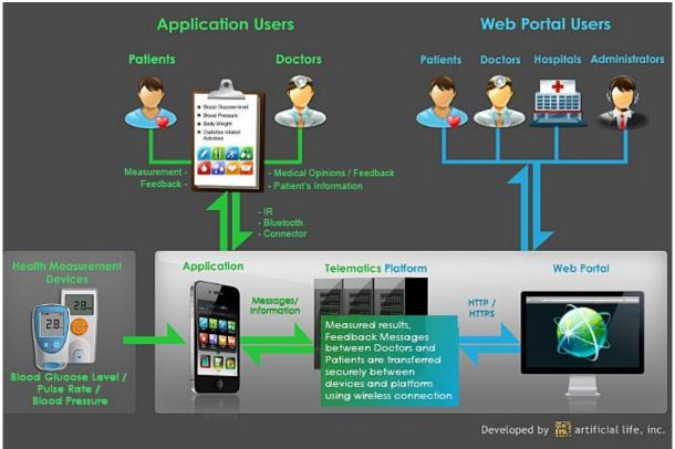
Figure 15: Architecture of GluCoMo
