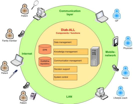
Figure 17: Functional architecture of a diabetes support system based on the MORE middleware
