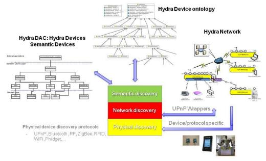
Figure 4: The 3-layered Discovery Architecture is part of the Hydra MDA.
