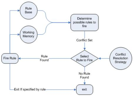
Figure 7: Forward Chaining (Proctor, et al., Drools Expert User Guide, 2011)
