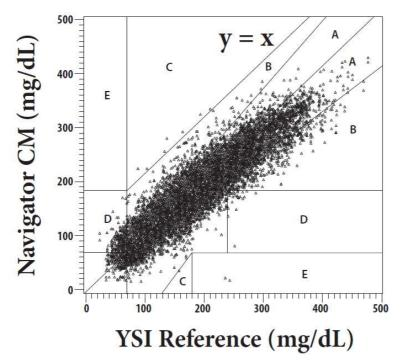
Figure 3: Clarke Error Grid, FreeStyle Navigator results compared to YSI results.
