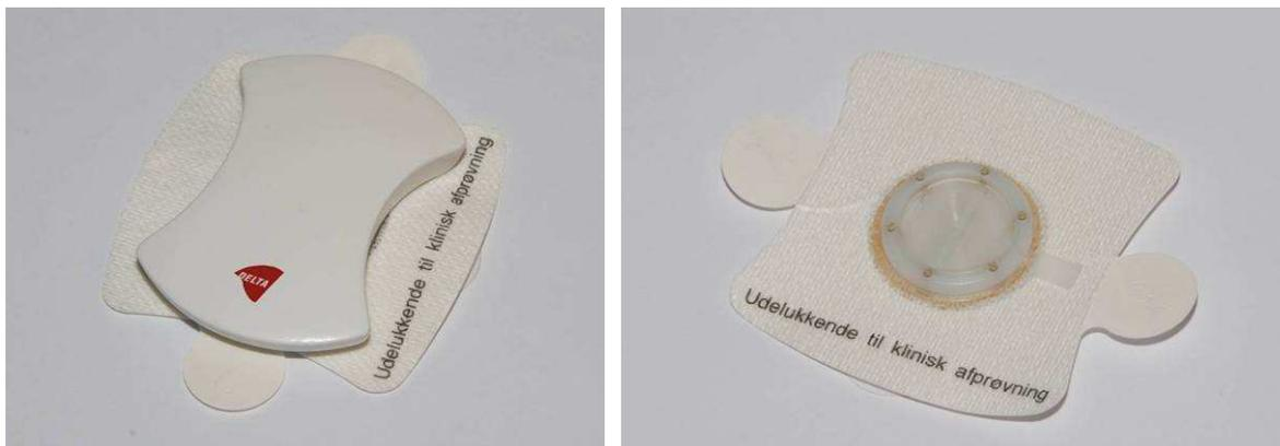
**Figure 4: The pictures show the ePatch. The left picture show the ePatch processor connected to an ePatch sensor. The picture to the right shows an ePatch sensor with the mechanical and electrical interface for connection to the ePatch processor.**
